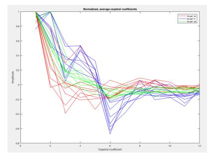
Figure 30: MFCCs for 8 separate recordings of the sounds \i\, \#\ and \a
