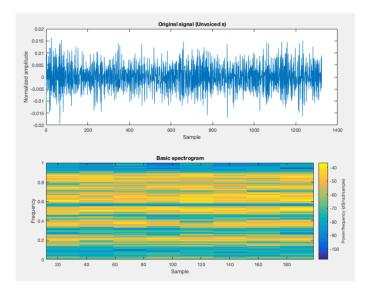
Figure 21: Single frame from an unvoiced 's' (time and frequency domain)
