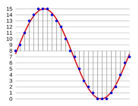
Figure 8: Sampling a waveform
