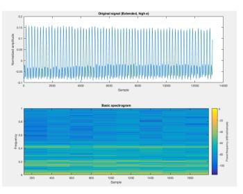
Figure 20: Single frame (extended) from the vowel 'e' (time and frequency domain)
