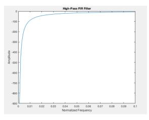
Figure 9: High-Pass FIR with a = .9
