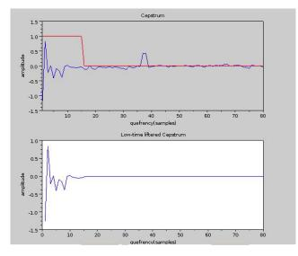
Figure 15: Example of Low-Time Liftering, [2]
