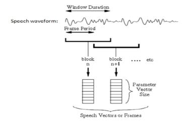
Figure 10: Windowing an audio signal, [23]
